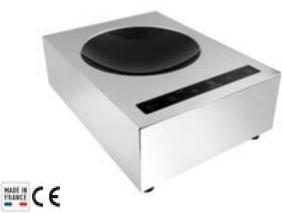
4-mm thick ceramic glass plate. 15-position thermostat. Suitable for intensive use in catering. Timer 99 minutes. Inductor diameter 280 mm. Suitable for 350 mm diameter woks.
