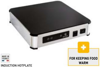
4-mm thick ceramic glass plate. 12-position thermostat. Interconnection system for up to 4 devices with a single power supply. Inductor diameter 180 mm. Interconnection lead sold separately. Suitable for use with Ø 120-360 mm containers.
